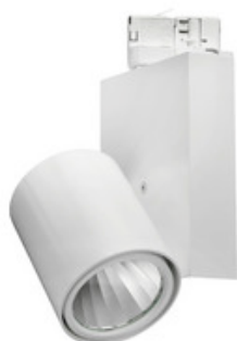
TC40388.00.56.51 LED Schienenstrahler dreh-schwenkbar, trackFFECT 5 DALI weiss 36W 40° 1800-16000K/RGB CRI90 TC40388.00.56.51
